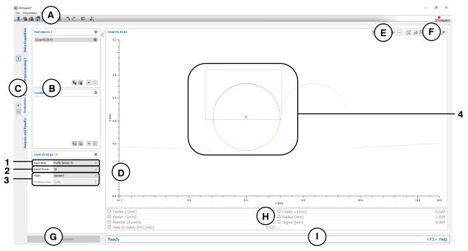
Fig. 6.20: "Circle Fit 2D" Measuring Program
