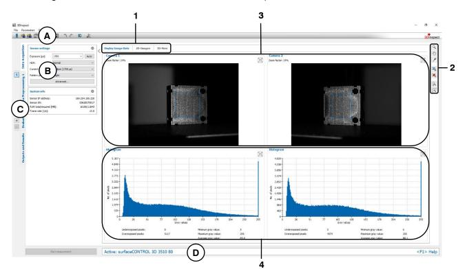
*Fig. 4.1: "Display Image Data" view (surfaceCONTROL/reflectCONTROL)*
