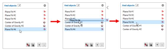
Fig. 3.53: Moving a measuring program
