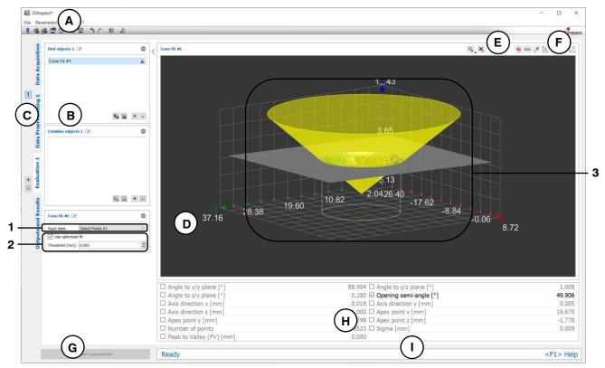
Fig. 6.8: "Cone Fit" Measuring Program
