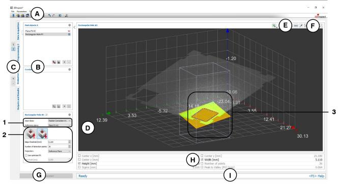
Fig. 6.11: "Rectangular Hole" Measuring Program
