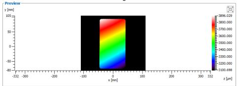
Fig. 3.8: Positioning the reference object - Distance too small
