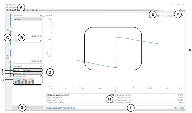
Fig. 6.28: "Gap 2D" Measuring Program
