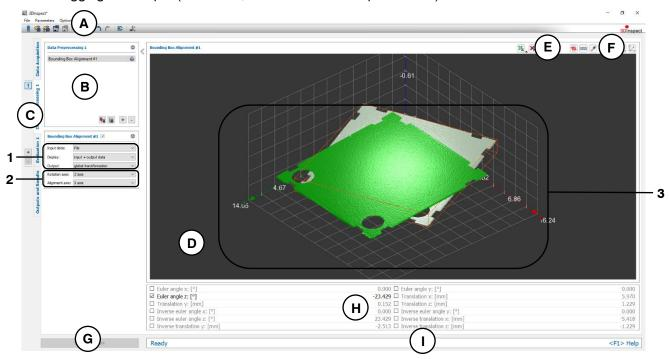
Fig. 5.5: "Bounding Box Alignment" Measuring Program
