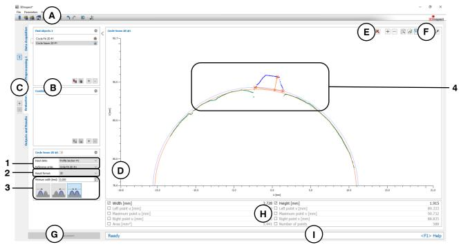
Fig. 6.26: "Circle Seam 2D" Measuring Program
