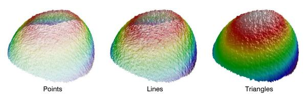
Fig. 3.40: Display methods for the 3D-View
