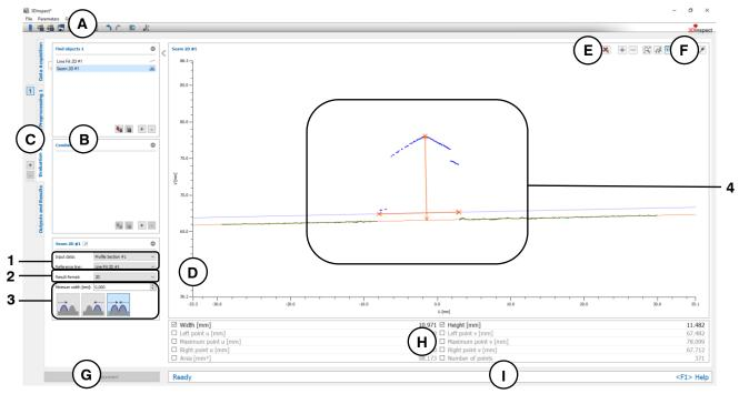
Fig. 6.24: "Seam 2D" Measuring Program
