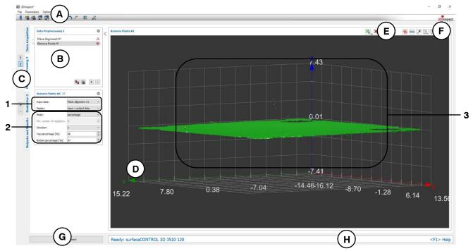
Fig. 5.20: "Remove Points" Measuring Program
