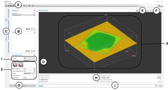
Fig. 6.12: "Rectangular Pad" Measuring Program
