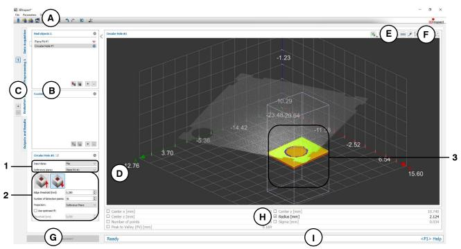
Fig. 6.9: "Circular Hole" Measuring Program
