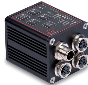
Fig. 11 Electrical connections on colorSENSOR CFO200
