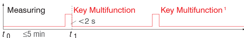
Fig. 64 Flow chart for zeroing, mastering (key Multifunction)
