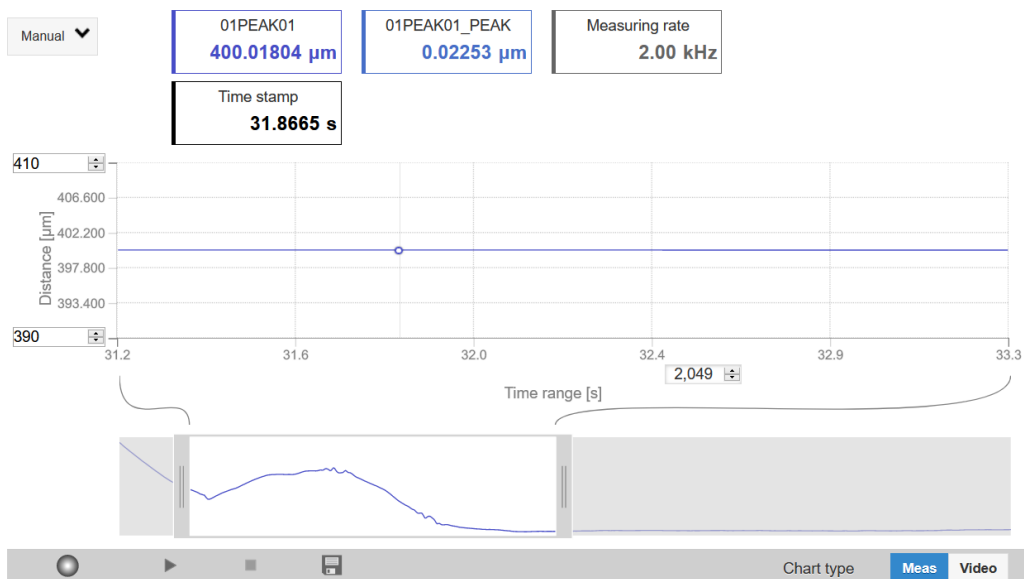
Fig. 76 Offline analysis of measured thickness results based on a one-sided thickness measurement
