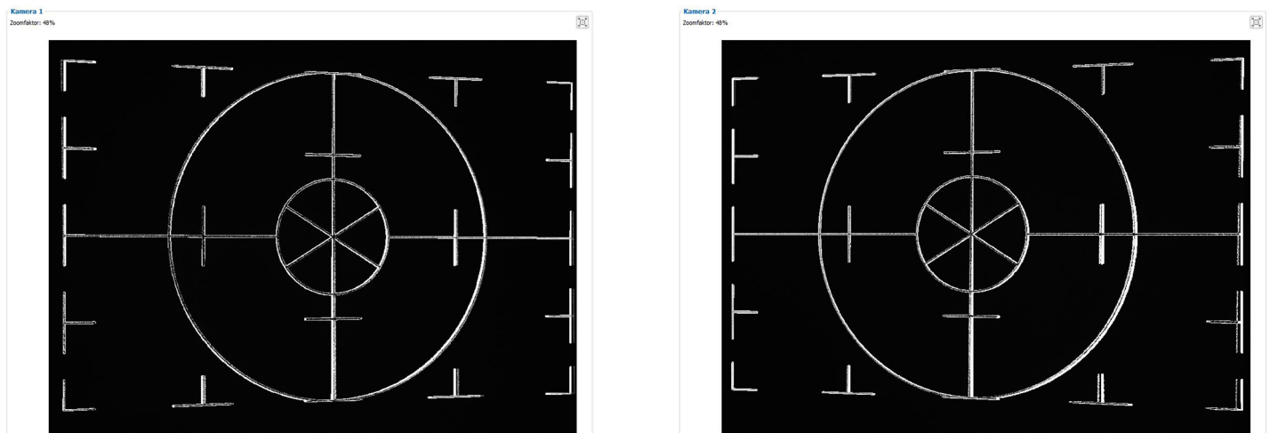
Fig. 22 Result of camera images when aligned with crosshair
