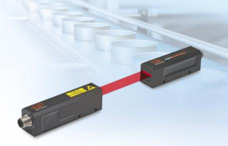
Light source and receiver can be mounted at any distance up to 5 m from each other. All models can be mounted both vertically and horizontally without additional brackets. The compact design of the housings and the 90° design allow the miniature micrometers to be mounted even in confined installation spaces. In addition the analog output, an adjustable limit switch is included. This can be operated in NPN (light switching) as well as in PNP logic (dark switching).
