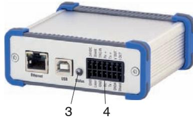
Fig. 7 Pin assignment 14-pin terminal block (4), type WAGO with view on pin *Laser*
