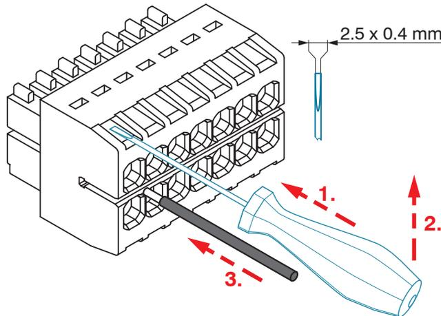
Fig. 39 Steps for wiring the cable clamp
