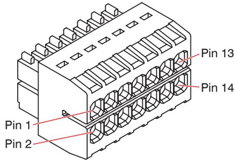
Fig. 38 Pin assignment 14-pin terminal box, type WAGO 713-1107
