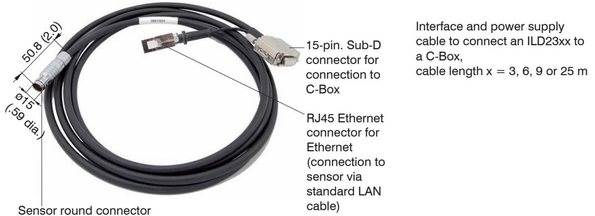
*Fig. 40 PC2300-3/C-Box/RJ45 power supply and interface cable*
