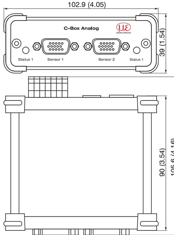
Fig. 1 Dimensions C-Box, dimensions in mm (inches), not to scale
