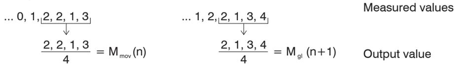
**i** Moving average in the controller C-Box allows only potentials of 2 for N. The highest averaging value is 1024.
