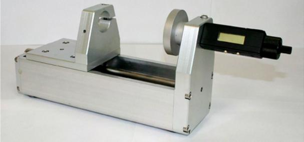
A silver, rectangular metal calibration device with a digital display and a micrometer head. It is designed for setting and adjusting the zero of sensors.        | Digital micrometer calibration device, setting range 0 - 25 mm, adjustable zero, for all sensors |
