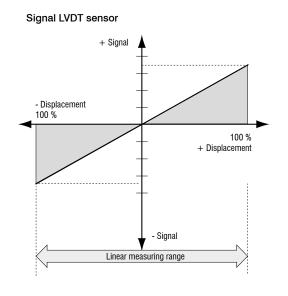
Measuring principle gauging sensor
