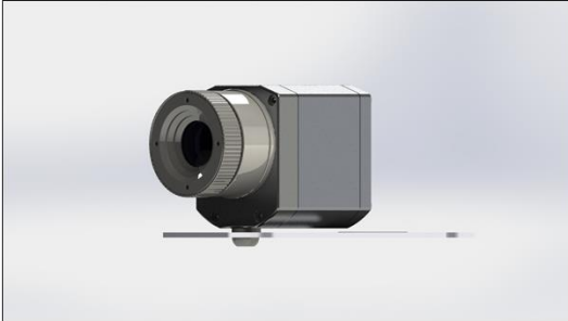
Figure 15: Fully assembled TIM camera on mounting
