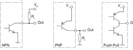
The switching behavior (NPN, PNP, Push-Pull) is programmable. The NPN output is, for example, suitable for adaptation to a local TTL logic circuit with auxiliary voltage of  $V_{ij} = 5 \text{ V}$ .
